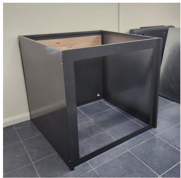
5. Centre box to ensure square and place lid on top; tap bolt & washer in place
