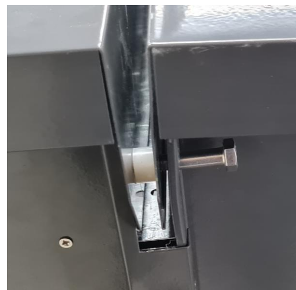
20. Insert bolt through lid 1, join channel, then into washer
