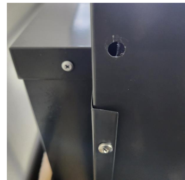
8. Sides now connected to wall strips/bridges
