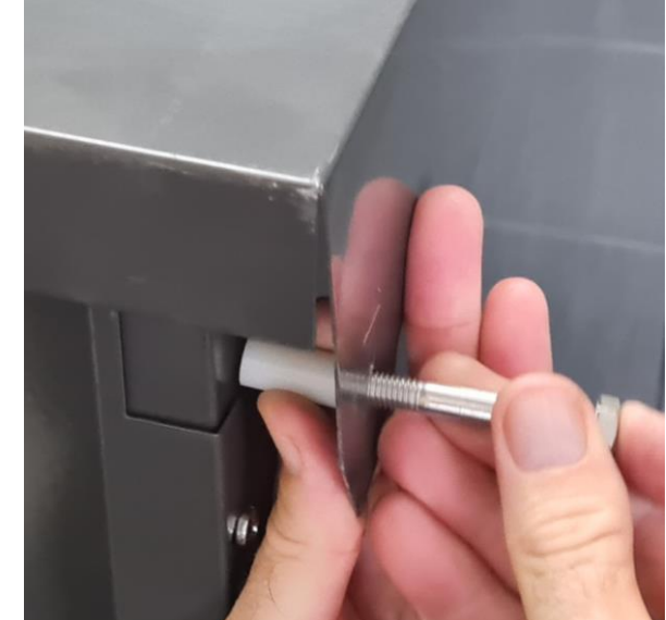
16. Insert large bolt through lid, then through washer, and into side panel
