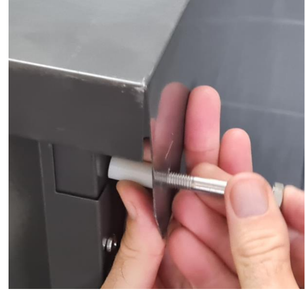
16. Insert bolt through lid, then through large washer, and into (larger) side panel
