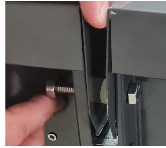
20. Insert bolt through joint channel and 2 nd lid, secure with nut
