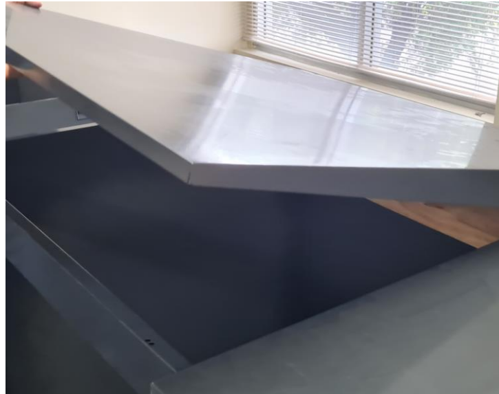
18. Position 2 nd lid and ensure square with box – if space is difficult, do after step 19
