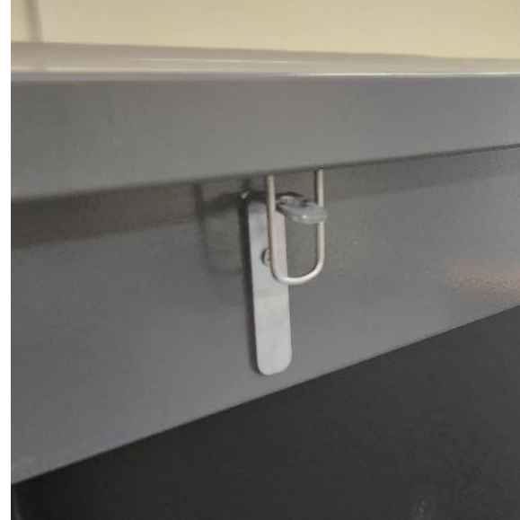
24. Screw latch onto front panel
