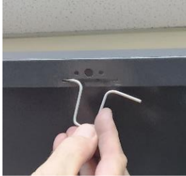
23. Insert latch hook into underside of lid
