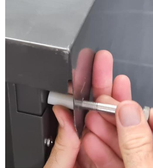
9. Tap bolt & washer in place; tighten nut
