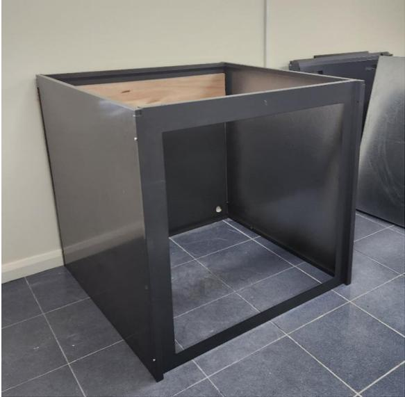
8. Centre box to ensure square and place lid on top; tap bolt & washer in place
