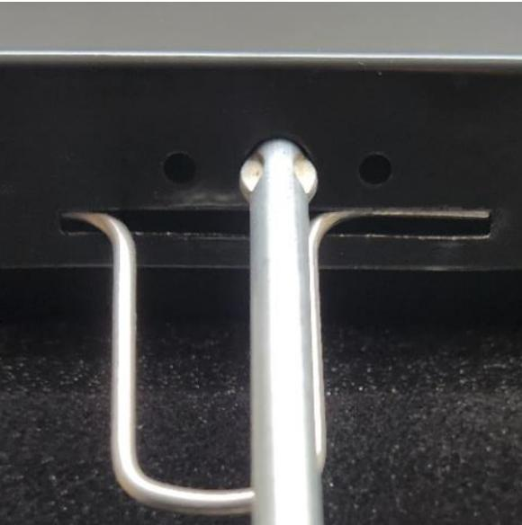
**18. Insert door stay into hole in underside of lid to hold open**
